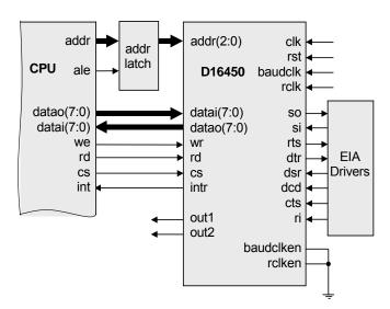
Typical D16450 and processor connection is shown in figure above.
